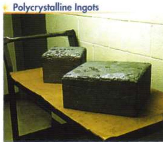
Figure 5-6. Polycrystalline silicon wafers are sawn from cast rectangular ingots.
